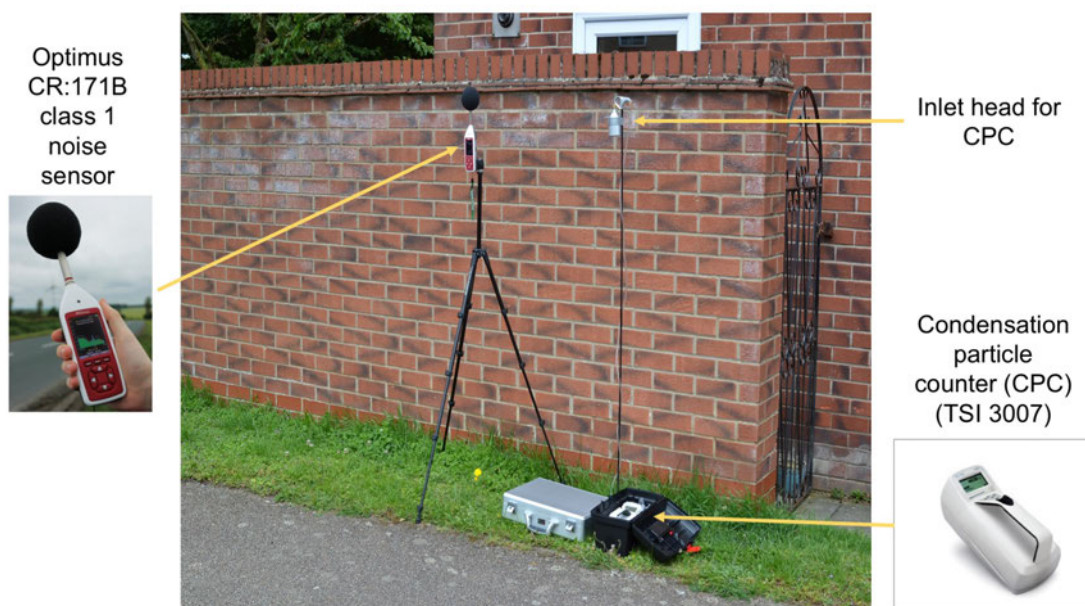
Figure 2: Typical setup for noise and UFP measurements
