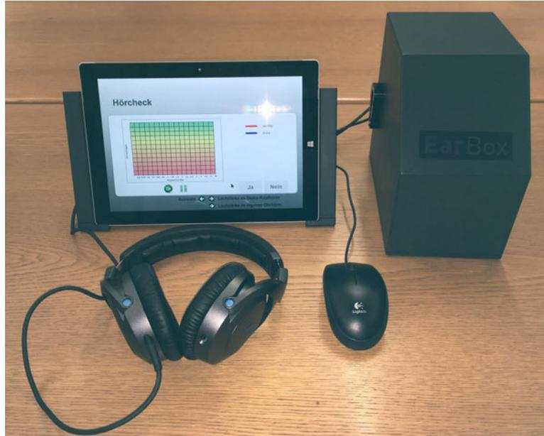
**Figure 4:** Suva’s Audio Demo Module with the EarBox containing the coupler for earphones
