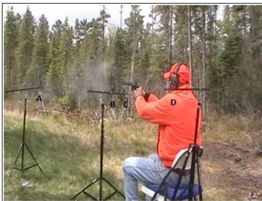
Figure 3: Microphone locations; A) 1.5 meters in front of muzzle, B) left of muzzle, C) left of chamber/cylinder and D) shooter's left ear with 5 cm offset from the skull. All other offsets were 10 cm left of the barrel.
